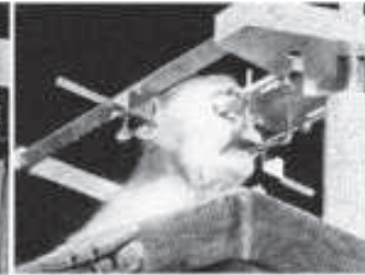
LAB-TRONICS stereotaxic instrument for monkey research. Adjustments for monkey investigation are similar to those used with cats. Ear plugs are usually necessary for work on monkeys and they are available with the instrument.
